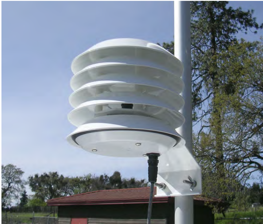
BX-596 Temperature/Pressure Sensor Installed on a BAM-1020 Inlet Tube
