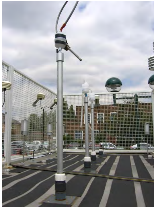
Figure 19: BX-302 zero filter during application in the field
