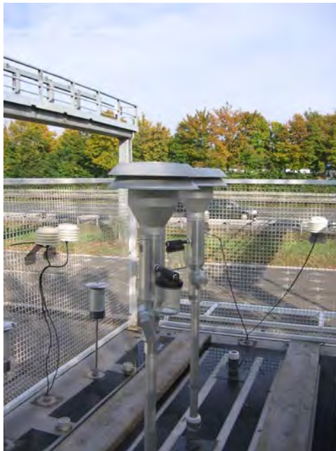
Figure 5: Sampling inlet BX-802 + SCC BX-807
