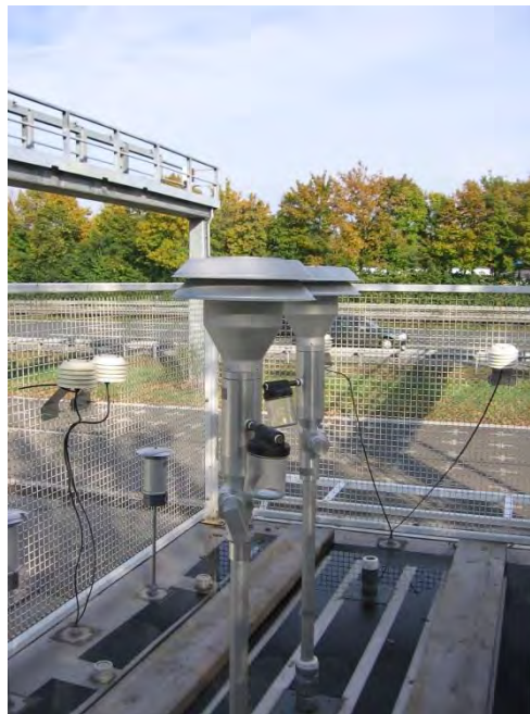
Figure 5: Sampling inlet BX-802 + SCC BX-807
