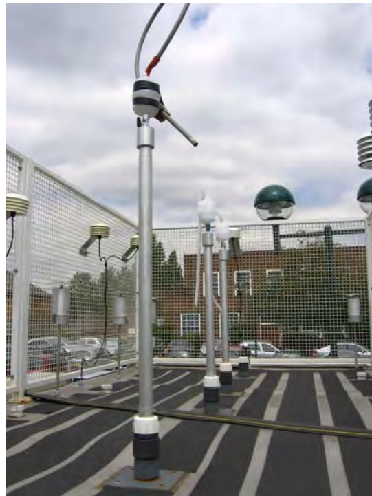
Figure 20: Zero filter BX-302 during field application
