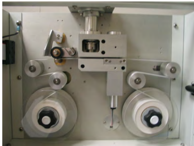
Figure 10: Front view BAM-1020, front cover opened
