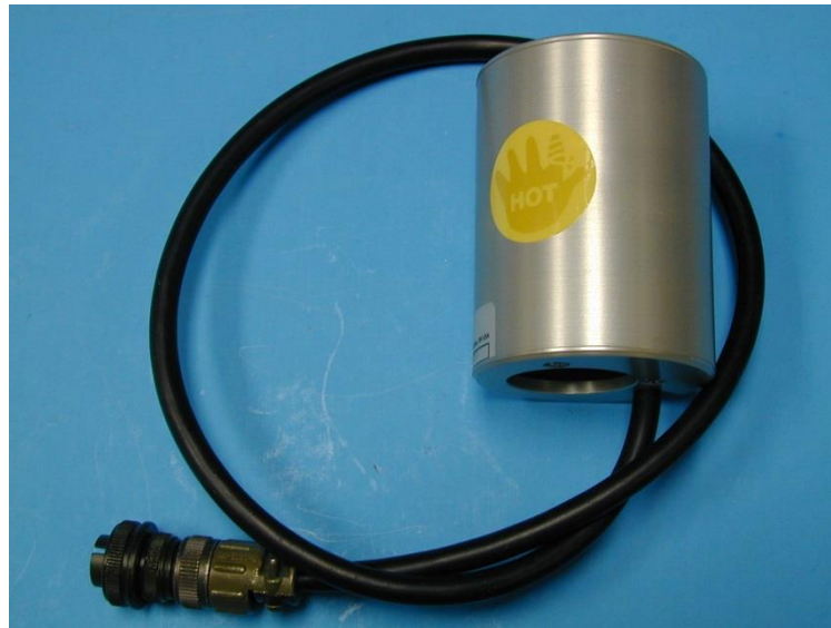
Figure 6: BX-830 sample heater
