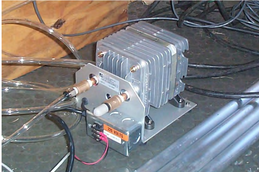
Figure 9: BX-127 vacuum pump
