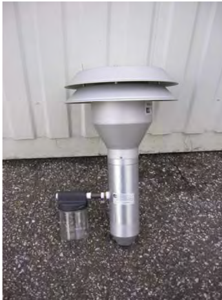
Figure 3: US- PM-sampling inlet BX-802 for BAM-1020
