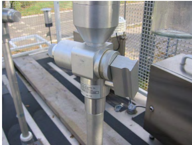
Figure 4: Sharp Cut Cyclone SCC BX-807 for BAM-1020
