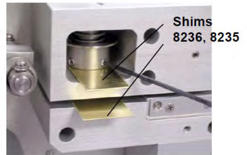
Using Shims for Reassembly
