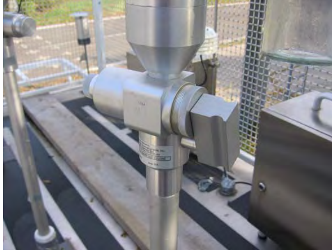
Figure 4: Sharp Cut Cyclone SCC BX-807 for BAM-1020
