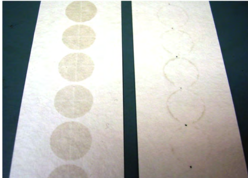
APDA-371 hourly filter tape spots
