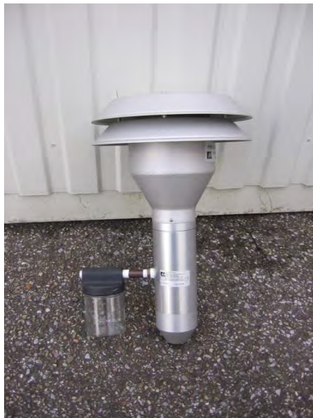
Figure 3: US-EPA PM 10 sampling head BX-802 for BAM-1020
