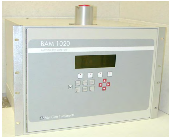
Figure 7: BAM-1020 measuring system
