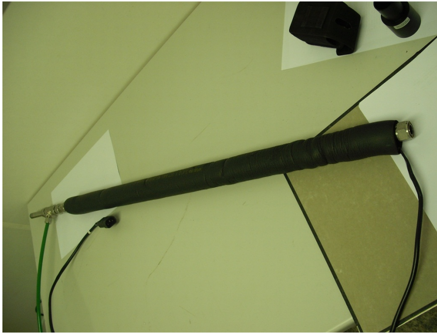
Figure 5: Heated sampling tube (DHS)
