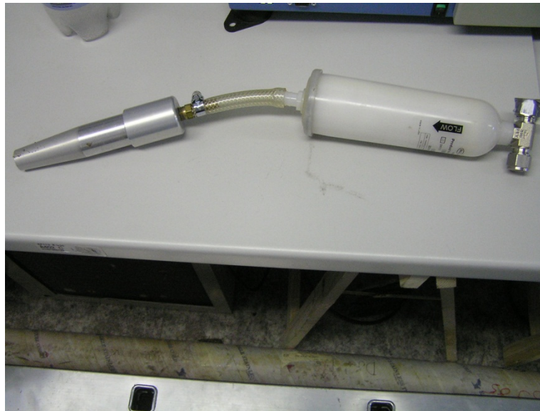
Figure 11: Zero filter for supplying air free of suspended particles and its connection adapter
