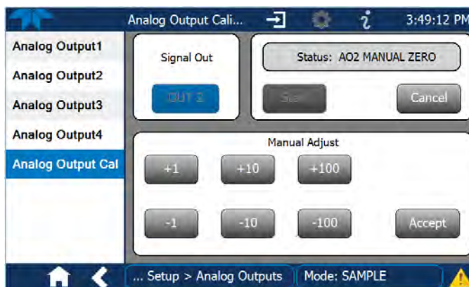
Figure 2-51. Analog Outputs Manual Calibration Screen (AO2 Example)
