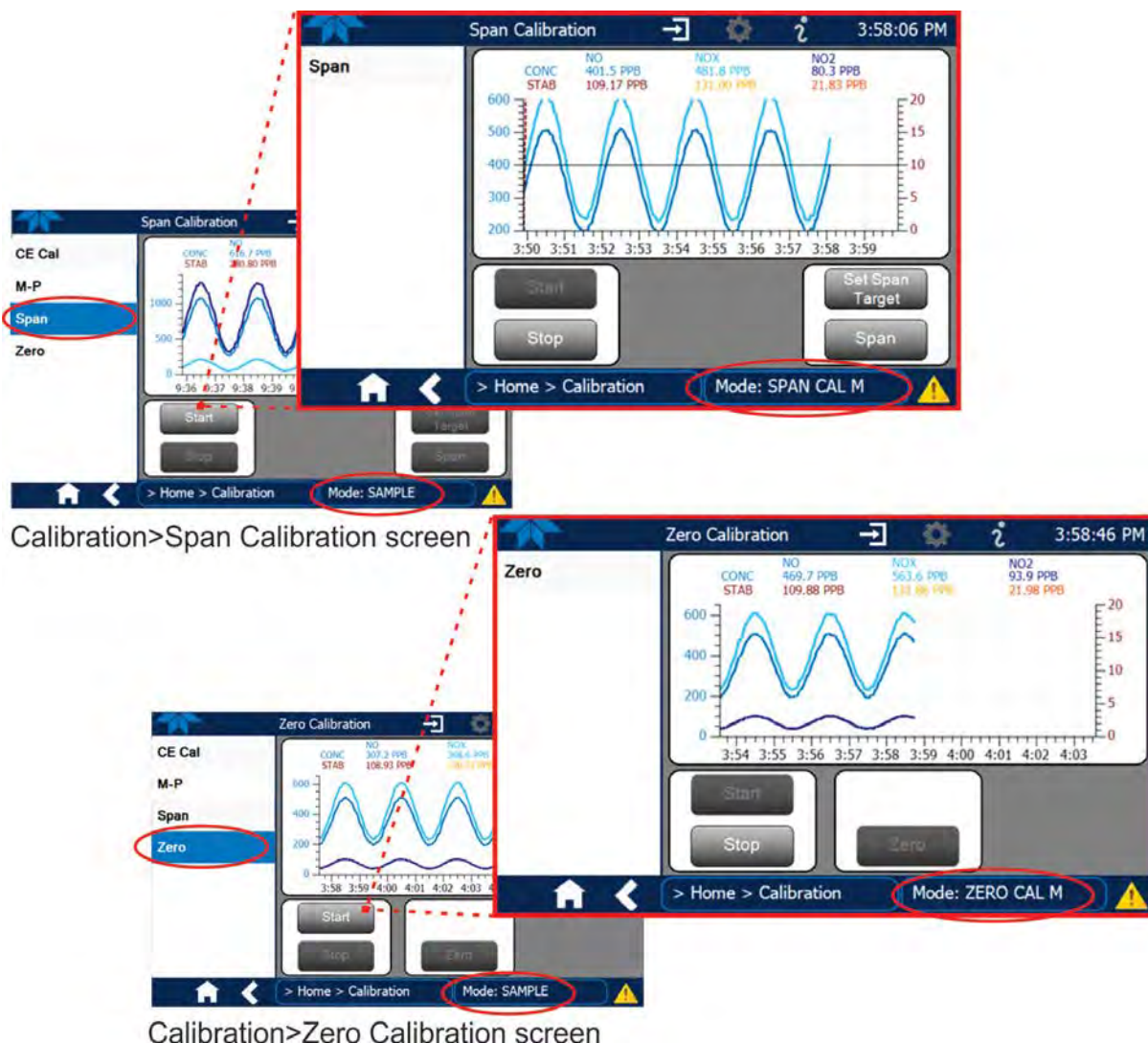
Figure 4-2. Zero and Span Calibration Screens
