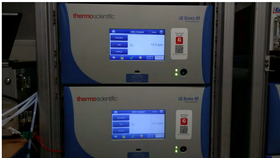
Figure 6: Tested 49iQ instruments with measured value display
