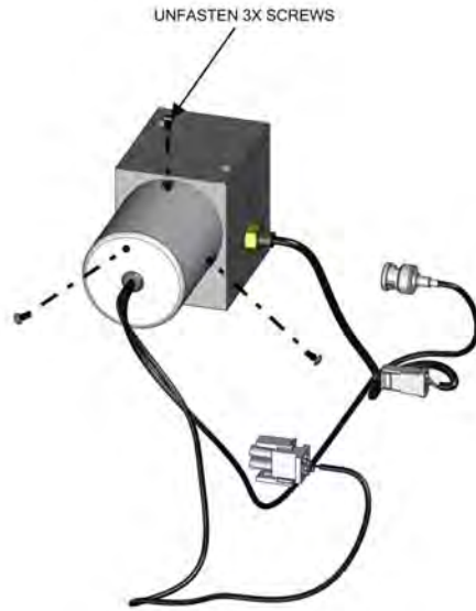
Figure 7-38. Removing the PMT Cover
